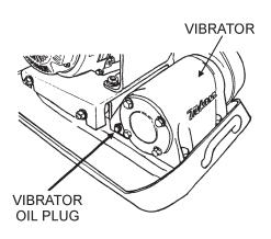
Figure 10. Vibrator Oil Plug
